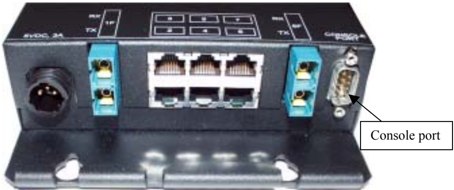
Fig. 2.2.2 Front View of Magnum mP62, Console port is located on the extreme right of the Hardened Switch
